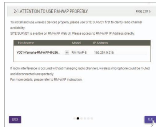
If no device information appears in the list, recheck the LAN cable connections. /
